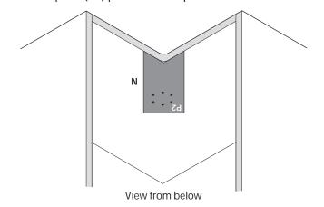
Insert carousel frame into base unit and align top and bottom mounting discs with pilot holes. When the runners are extended, there should be an equal distance on both sides between the runner and the cabinet side.
