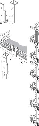
IMPORTANT - The unit has a maximum loading limit of 100kg. Load should be evenly distributed across all trays with maximum load capacity for each tray not exceeding 16kg.
