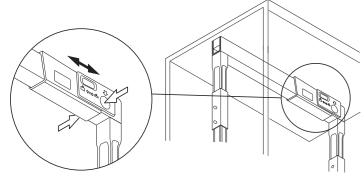
Now refer back to instruction No. 7 and check the distance is still 61mm front and back. If not, release grub screws C01 and make the necessary adjustments. **12** Adjust the horizontal and lateral door alignment with screws on the door brackets.
