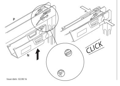
4 Insert the top into the bottom frame, and then attach this assembly to the bottom runner.
