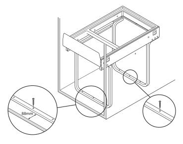
2 Before permanent attachment to the cabinet base, fit containers and lid and test for ease of opening and container removal. Ensure the unit is clear of door hinges and other obstructions during operation.
