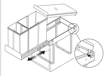
Attach the four brackets to the cabinet base using x4 short screws and x1 long screw to each bracket.
