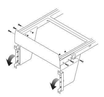
**2** Measure 56mm from the cabinet front face and position the frame allowing for any obstruction from above or the sides. Fit the two long screws through the central holes
