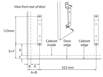
Fit the detached brackets to the door using the vertical measurements X+Y and the horizontal measurements A+B to locate.
