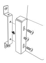
Reattach the inner brackets to the door brackets
