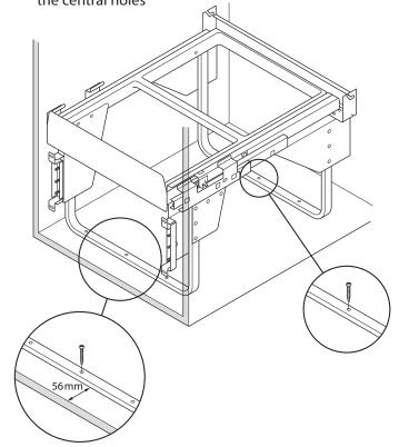
Before permanent attachment to the cabinet base, fit containers and lid and test for ease of opening and bin removal. Ensure the unit is clear of door hinges and other obstructions during operation.
