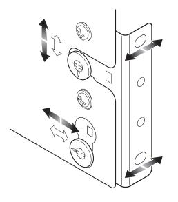
Important - The unit has a maximum loading limit of 30kg including door.
