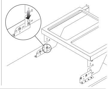
**7** Fold the door up to its vertical position, engaging the upper lugs with the slots on the frame. Secure this in place with the M6 x 10mm screws.
