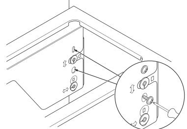
8 Use the adjustment screws to align the door.
