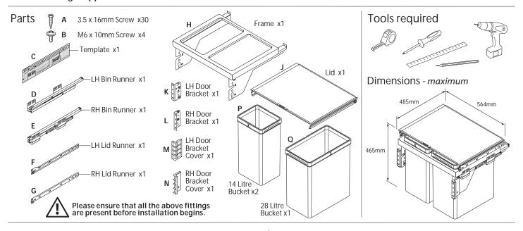
Mark a line 430mm up from the internal cabinet base. Position the template on this line and mark screw positions.
