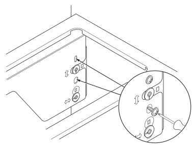
**8** Use the adjustment screws to align the door.
