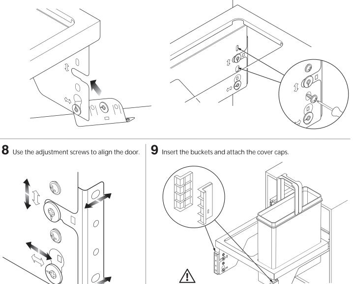
IMPORTANT - The unit has a maximum loading limit of 30kg including door.
