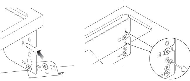
**8** Use the adjustment screws to align the door.
