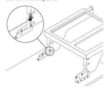
7 Fold the door up to its vertical position, engaging the upper lugs with the slots on the frame. Secure this in place with the M6 x 10mm screws.
