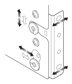
**9** Insert the buckets and attach the cover caps.
