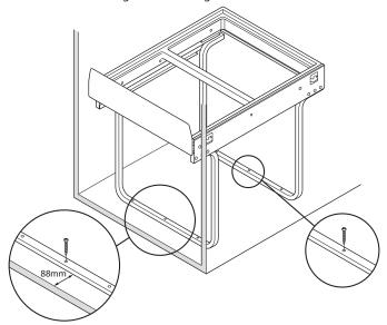
Before permanent attachment to the cabinet base, fit containers and lid and test for ease of opening and container removal. Ensure the unit is clear of door hinges and other obstructions during operation.
