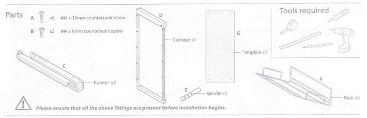
Mark screw positions for runners on right hand side of cabinet or use the installation template included.
