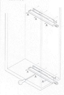
3 Slide carriage onto runners ensuring the carriage sits under the back retaining lugs. Fully extend carriage and secure to top and bottom runners using screws (B).
