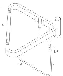
**4** Assemble the components onto the support pole ensuring a rod is inserted below each bush at the appropriate height.
