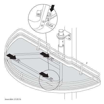
Position the tray opening bracket beneath the opening rail and screw to the door - recommended that this be fitted on the centre line of the door.
