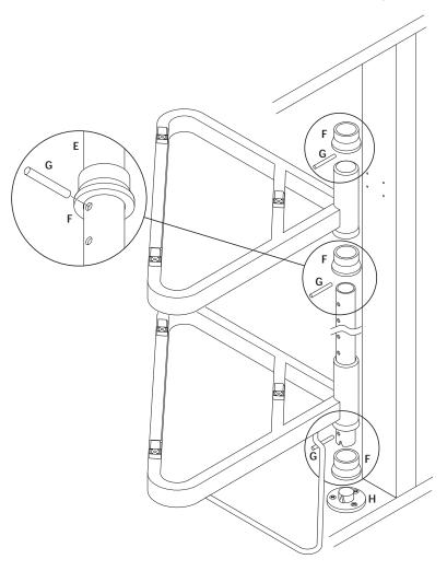
Fit the top bracket to the pillar. Push bung into top of support pole.
