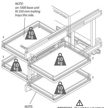
NOTE: on 1000 base unit fit 300 mm leading trays this side.
