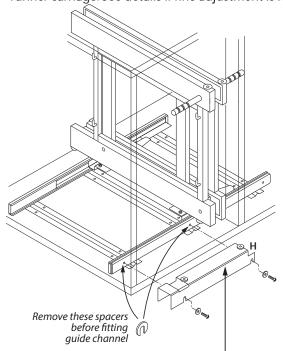
IMPORTANT: The guide channel height must be carefully adjusted to allow unrestricted forward movement of the Optimiser and to ensure the limit stop is held by the nylon wheel.
