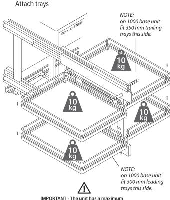
loading limit of 40kg. Load should be evenly distributed across all trays with maximum load capacity for each tray not exceeding 10kg.
