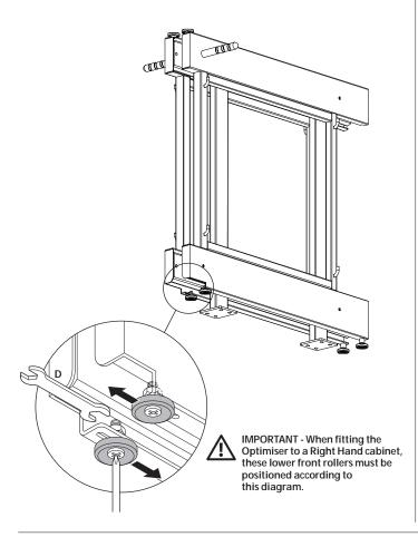
Lower slider unit onto runner carriage and attach the 6 nuts.
