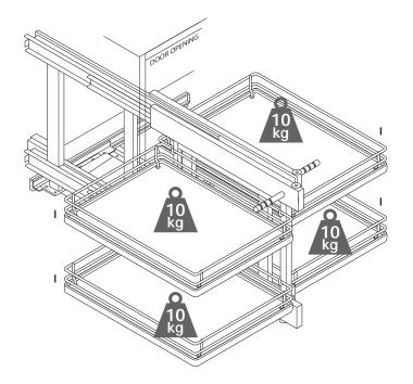
IMPORTANT - The unit has a maximum loading limit of 40kg. Load should be evenly distributed across all trays with maximum load capacity for each tray not exceeding 10kg.
