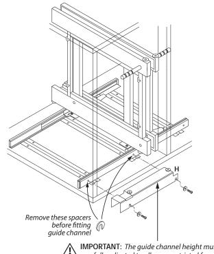
IMPORTANT: The guide channel height must be carefully adjusted to allow unrestricted forward movement of the Optimiser and to ensure the limit stop is held by the nylon wheel.
