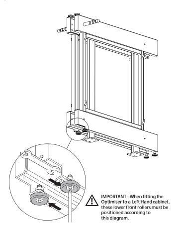
Lower slider unit onto runner carriage and attach the 6 nuts.
