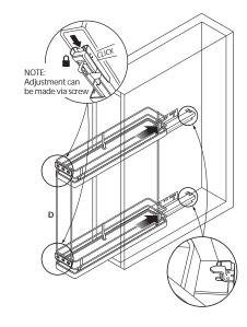
**3** Secure brackets to inside face of door. Using template G.
