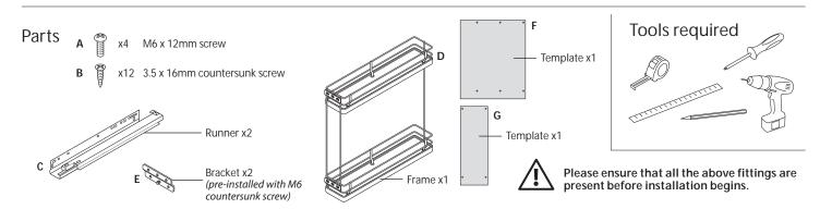
**1** Fit runners to left hand side of cabinet. Using template F.
