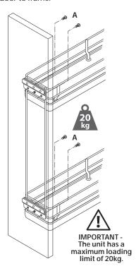
**5** Adjust the door using the screws as shown;
