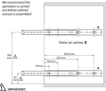
Dimensions are based upon a 18mm thick carcass. For other carcass thickness, adjust accordingly.
