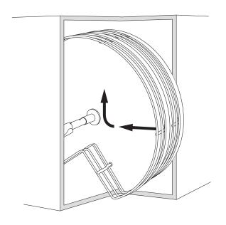
Locate the pole on the bottom mounting plate ensuring the lug is engaged. Extend the pole so that the top mounting plate is trapped.
