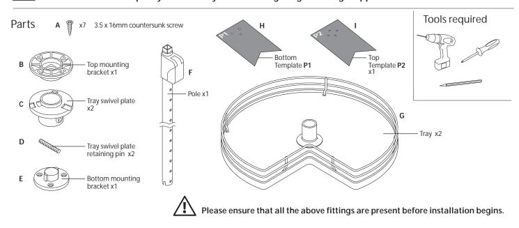
Mark base of cabinet for fitting carousel using the template (P1) provided. Drill pilot holes. Fit bottom mounting bracket using 3 screws.
