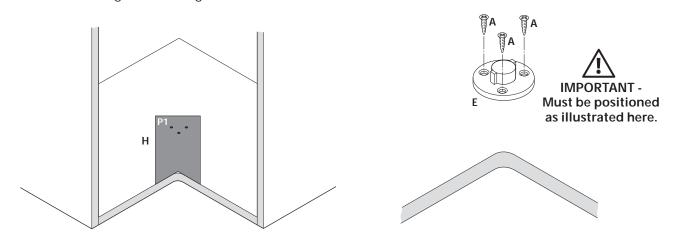
Mark top of cabinet for fitting carousel using the template (P2) provided. Drill pilot holes. Fit top mounting bracket using 4 screws.
