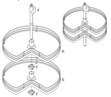
4 Lay the assembled unit on its side and insert into the cabinet. Rotate the unit so that the pole is vertical.
